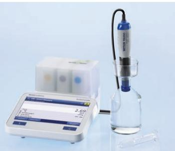
The biochemical oxygen demand (BOD) of any effluent can be readily checked with the InLab® OptiOx sensors. With the special BOD adapter, the sensors can be fitted to all current types of BOD bottles. According to the EPA (Environmental Protection Agency, USA), stirring is not necessary when using our OptiOx sensors.
